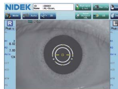
Reflected image of double mire rings
